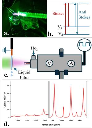
**Fig. 1.** (a.) Photograph of 532 nm light and plasma irradiating a liquid film (b.) Stokes and anti-Stokes Raman scattering energy level diagrams (c.) Schematic of image in (a.) (d.) anti-Stokes cyclohexane spectrum (left) and Stokes cyclohexane spectrum (right).
